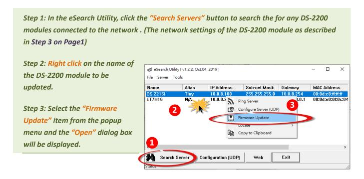
Step 4: In the "Open" dialog box, select the firmware file (DS2200.dat) that will be used to update the module and then click the "Open" button.
