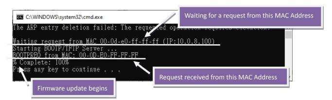
Note: If the Remote Firmware Update method fails, please refer to Section 3.1 Firmware update in BOOT mode (local operation) to restore the module.
