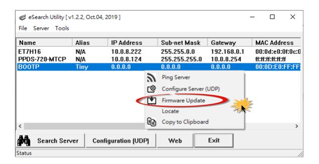
Step 5: Refer to Steps 4 to 17 in "Chapter 2-Firmware Update Procedure" to complete the update process. Note, the module will response with no IP address in the BOOTP mode. User has to assign a valid IP manually in step 5 of page 3.
