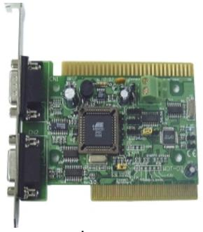
The WDT-03 is a advance watchdog timer & monitoring, WDT, designed for ISA/PCI bus or any bus with RS-232 port. After the watchdog timer is enable, the WDT-03 will monitor the operations of software and hardware in the most inexpensive cost. It will reset the CPU if there is any software or hardware problem.
