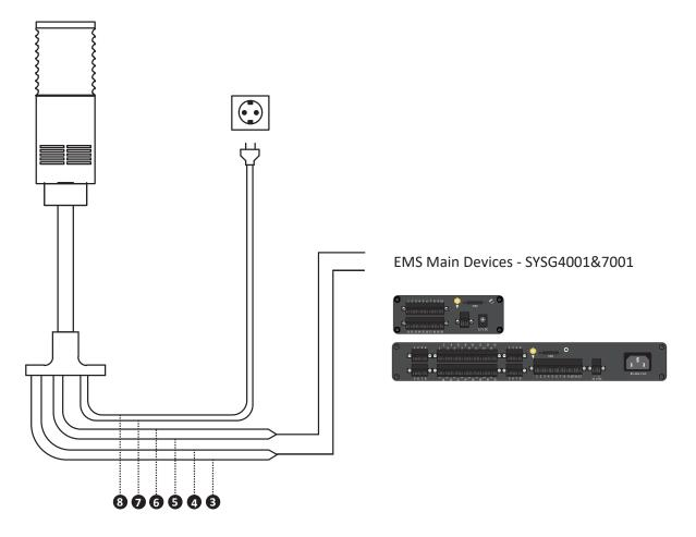
SYSGAC13 Signal Tower can be connected to SYSGuard 7001&4001 EMS Devices directly.
