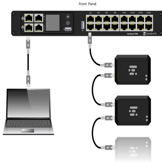
Exagate sensors can be cascaded. The top left RJ45 input on the SYSGuard device can be used to set up sensors and dry contact modules (see above).
