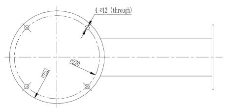
Figure 2.3.1.3 Front view of Wall-mounted Bracket
