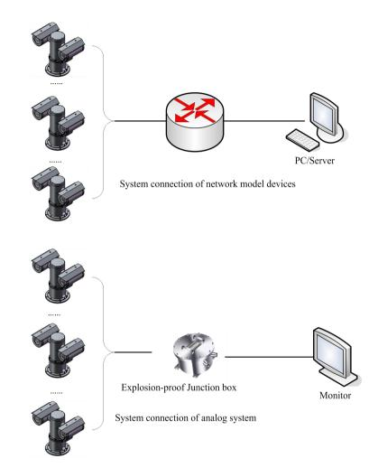
Figure 2.5.1 System connection
