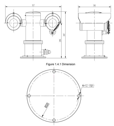
Figure 1.4.2 Distribution of installation holes
