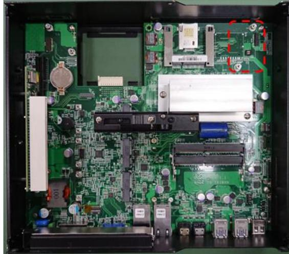
2. Insert the female connector of PoE daughter board to the male connector on system motherboard.
