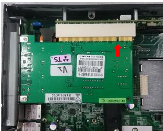
5. Fasten one screw to secure the PCI(e) expansion card.
