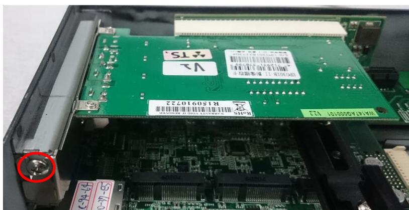
6. Slide the clamp arm of retention module until it contacts the edge of PCI(e) expansion card.
