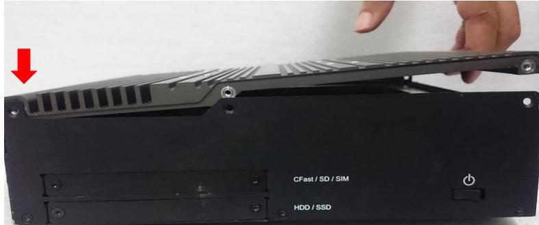
2. Fasten the six screws at front and rear panel to secure the top cover.
