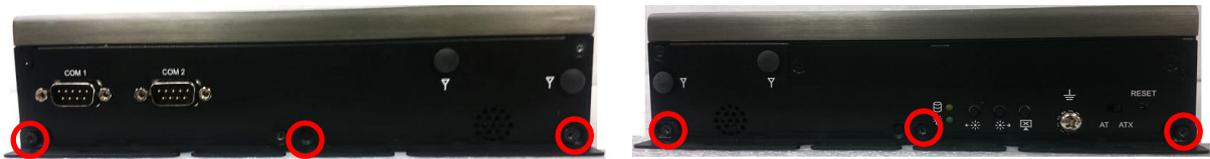
The following picture indicates six wall mounting holes at each side.
