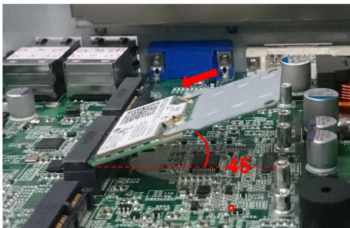
4. Press down the module and use the two screws to fix the module.
