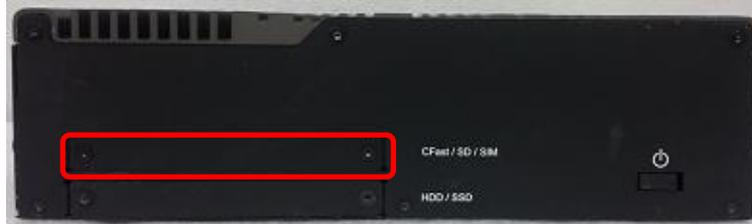
2. Loosen two screws to remove the cover plate.
