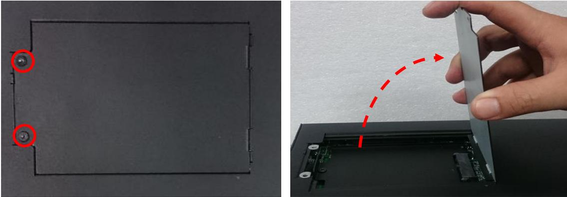
3. Loosen three screws and take the HDD bracket out of HDD compartment.
