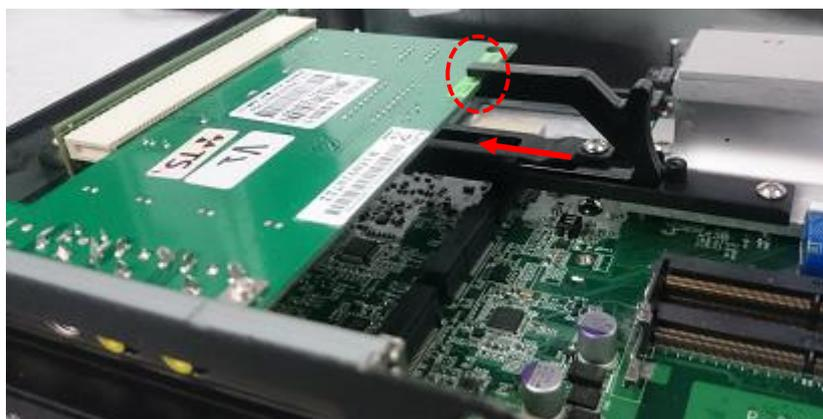
7. Finally, fasten the screw that were previously loosen halfway to fix the retention module.
