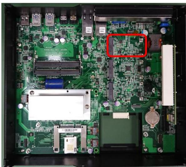
2. Tilt the Mini PCIe card at a 45-degree angle and insert it to the socket until the golden finger connector of the card seated firmly.
