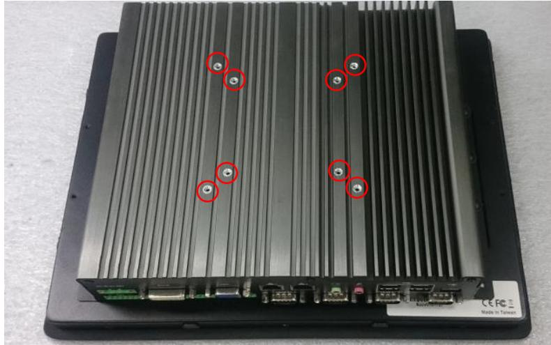
1. The following picture uses a panel PC (P2000+CV display module) as a demonstration. To attach the panel PC to a VESA stand, please fasten eight screws as indicated to fix it on the stand. (Please refer to section 3.16 in this manual for how to attach PC2000 to CV display module.)
