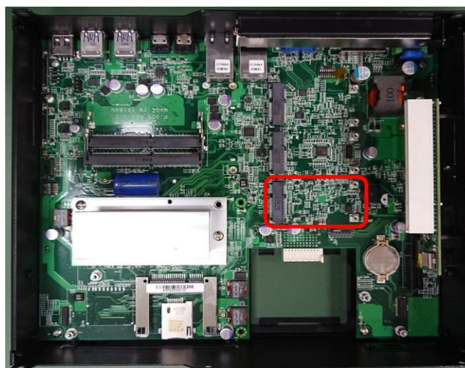
2. Tilt the mSATA card at a 45-degree angle and insert it to the socket until the golden finger connector of the card seated firmly.
