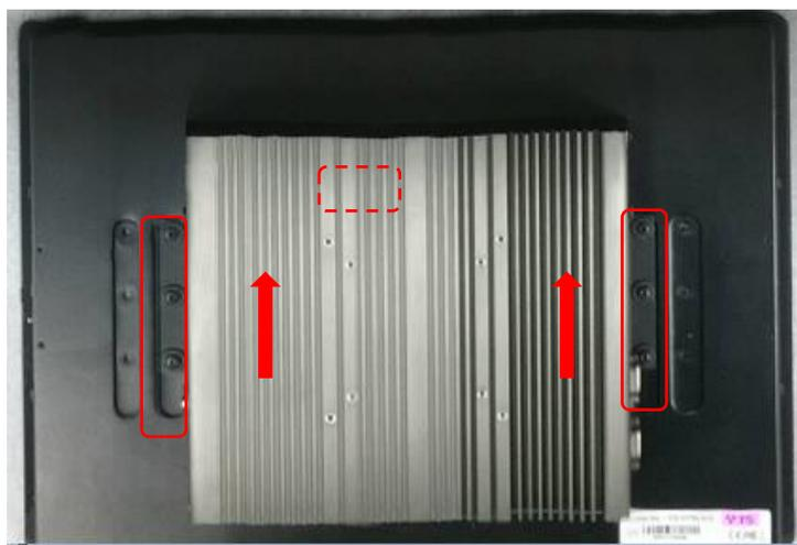
8. Fasten six screws to secure P2000 on the display module.
