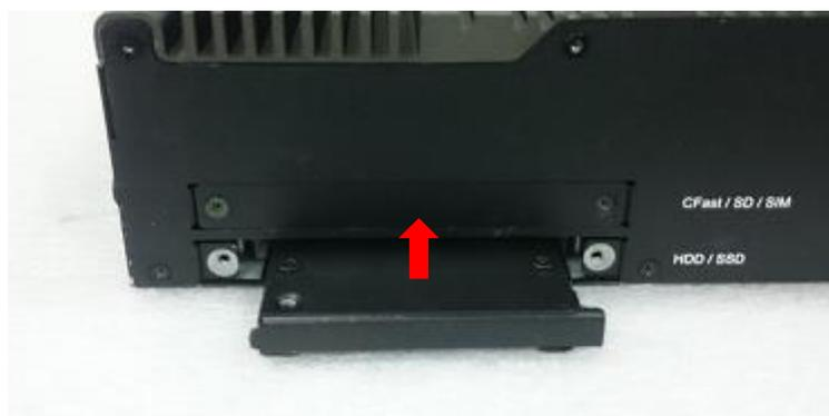
7. Put back HDD bay cover at front panel, and fasten it with two screws.
