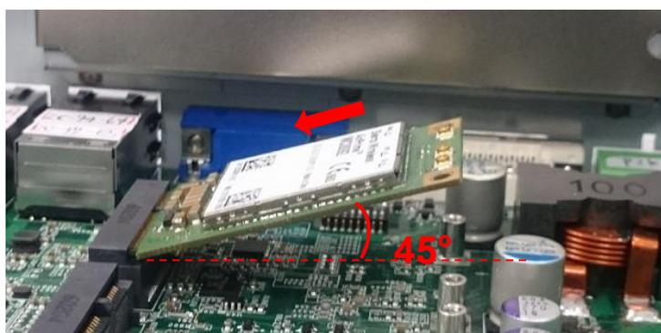
3. Press down the module and use the two screws to fix the module.
