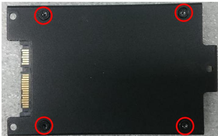
6. Secure the HDD bracket with three screws.
