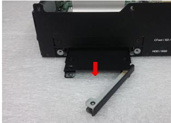
5. Place the HDD bracket on screw-hole side of HDD. Use four screws provided to assemble HDD on the bracket.
