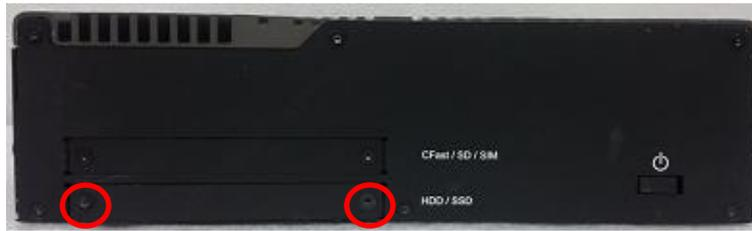
8. Fasten one screw to secure the HDD bracket on the system chassis.
