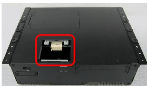
6. Place the P2000 on the display module through its display connector hole as indicated.
