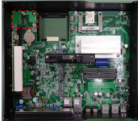
2. Insert the female connector of power ignition board to the male connector on system motherboard.
