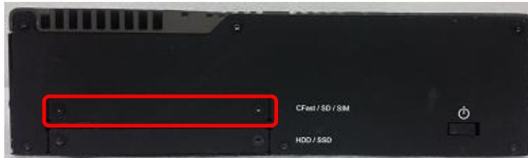
2. Loosen the two screws to remove the cover plate.
