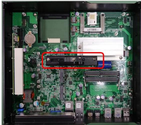
2. Loosen one screw halfway as indicated to have the clamp arm slidable.
