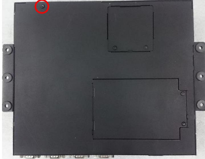
2. Loosen the two screws to remove the HDD bay cover bracket.
