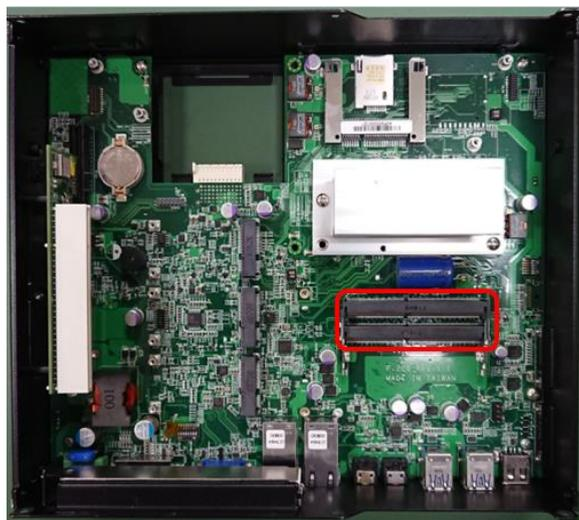
2. Tilt the SODIMM module at a 45-degree angle and insert it to SODIMM socket until the gold-pated connector of module contacted firmly with the socket.
