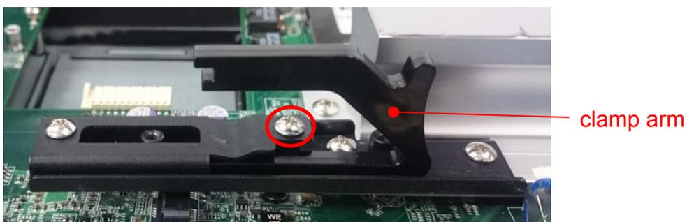
3. Loosen one screw to remove the PCI bracket.
