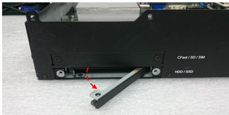
4. Hold the rotating arm to pull out the HDD bracket.
