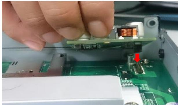
3. Fasten two screws to secure the PoE board.
