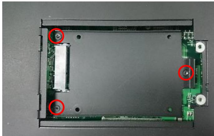
4. Place the HDD bracket on screw-hole side of HDD. Use four screws provided to assemble HDD on the bracket.
