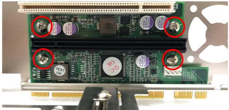
4. (1) Loosen the screw to remove I/O bracket. (2) Loosen the 2 screws halfway to allow the card retainer to be adjustable.
