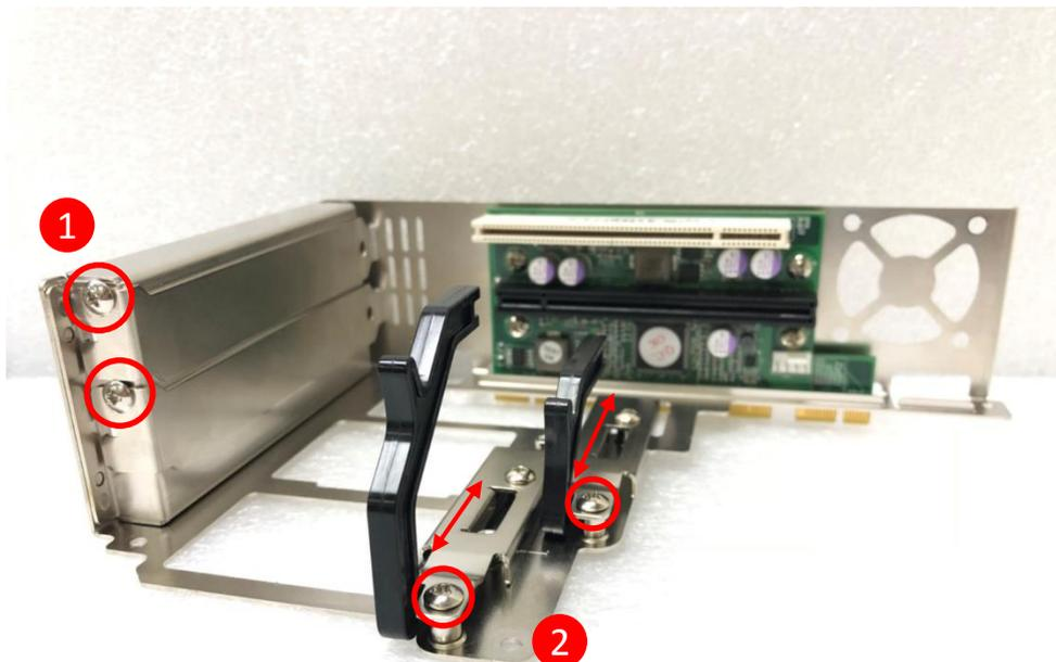
5. (1) Insert a PCI(e) add-on card to the slot. (2) Fasten the screw to secure it (3) Push the card retainer forward to against the edge of the add-on card. (4) Tighten the screw to fix the card retainer.
