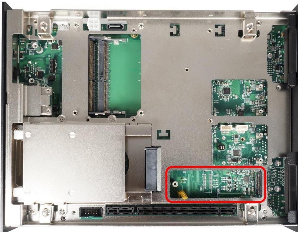
3. Tilt the Mini-PCle module at a 45 degree angle and insert it to the slot until the gold-pated connector of module contacted firmly with the slot.
