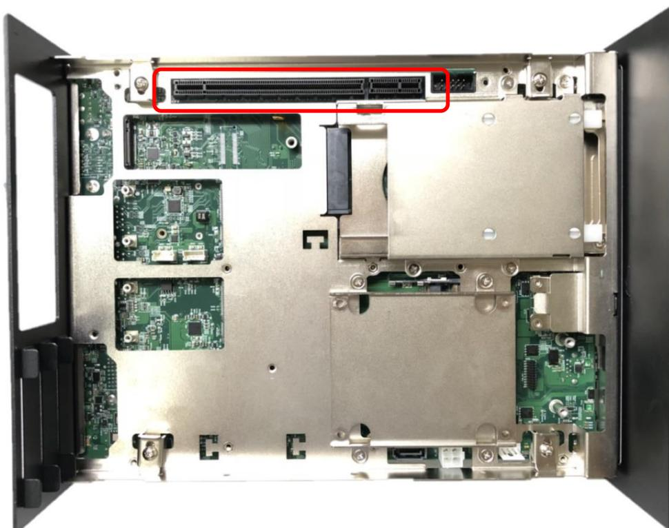
7. Install the module assembled in step 4 into the riser card slot, and fasten the 4 screws to secure it.
