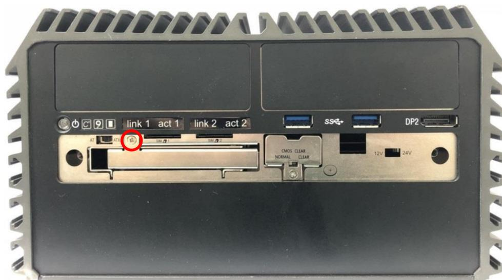
3. Move the rotating arm out and pull the HDD bracket out.
