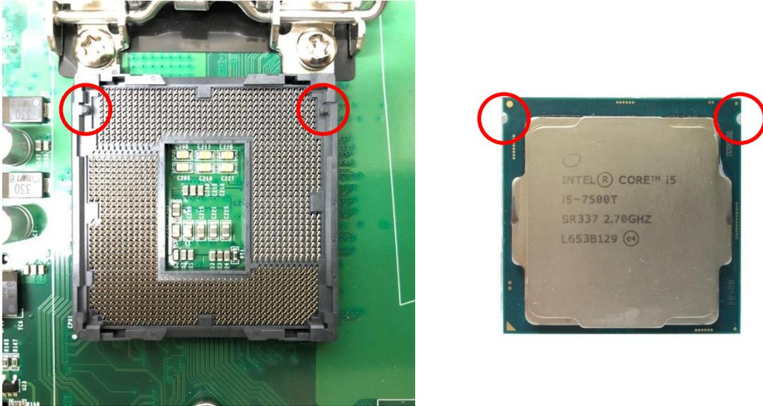
4. The notches of socket provide the space for fingers while lowering the CPU, hold the CPU by the edges toward the notches and insert the CPU gently.
