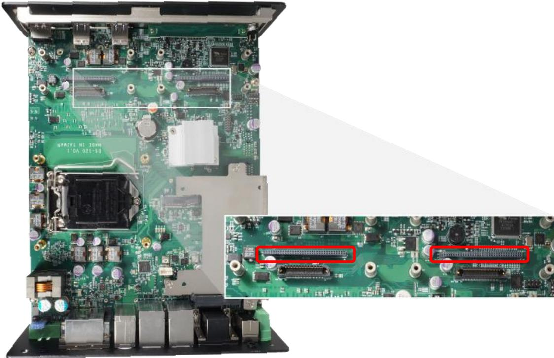
3. Insert the CMI module carefully into the CMI connector on main board.
