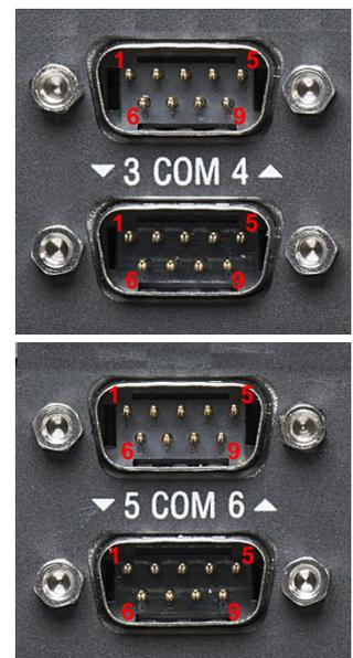
**Note: COM3/4/5/6 are isolated COM, each pin5 (GND) is independent.**
