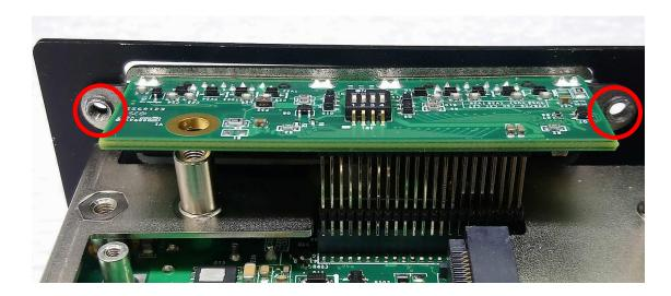
4. Push the connector pins on CMI-COM module until the pins can be inserted completely to the female connector (BTB\_FH2 or BTB\_FH1) on the system's mainboard.
