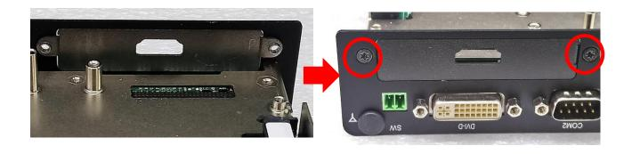
3. Align the hole on CMI-HD module with the screw hole on the system's mainboard module, and insert vertically to the female connector (BTB\_FH1) on the system's mainboard.
