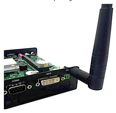
5. Attach the RF connector at another end of cable onto the module.
