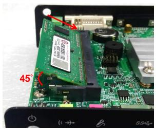
3. Press the module down until it's fixed firmly by the two locking latches on the sides.
