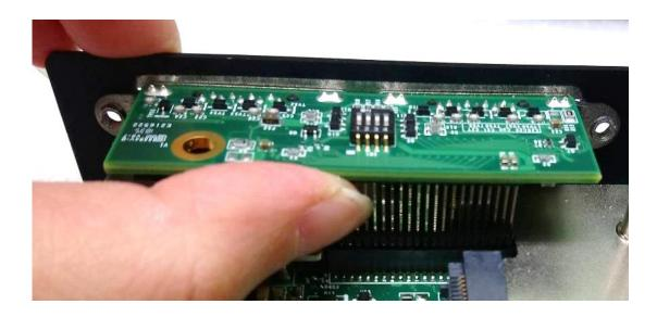
5. Make sure the hole on CMI-COM module is aligned with the screw hole on the system's mainboard, and fasten a screw to fix it.
