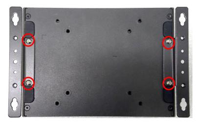
2. Fasten the screws through the bracket mounting hole to mount system on the wall.
