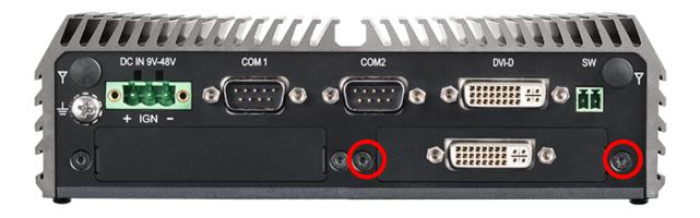
1. Unscrew 2 screws to remove bracket#3 from rear panel.
