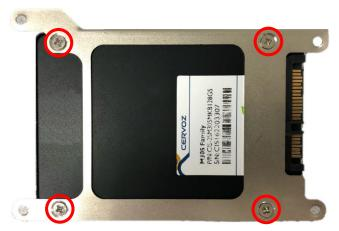
3. Turn over the HDD bracket. Connect the HDD bracket to the SATA connector of the unit and fasten the 4 screws.
