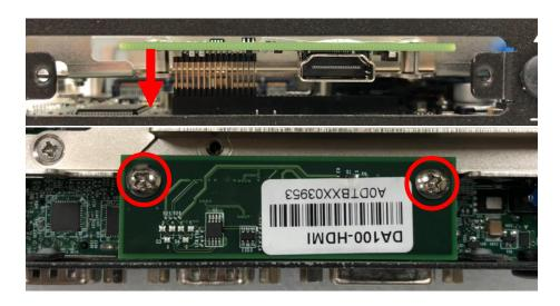
3. Attach the CMI-HD bracket, fasten 2 screws as marked on photo.
