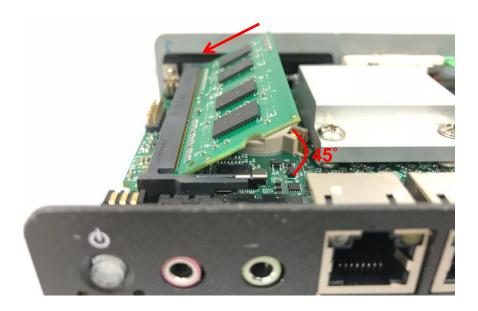
3. Press the module down until it's fixed firmly by the two locking latches on the sides.
