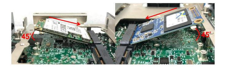
4. Press down the module and use the two screws to fix the module.
