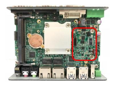
2. Insert the female connector of CFM-PoE module to the male connector on system motherboard.
