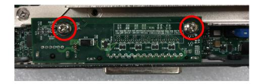
3. Attach the CMI-LPPS bracket, fasten 2 screws and 2 D-Sub jack screws as marked on photo.
