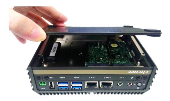
2. Fasten the 4 screws to fix the cover.
