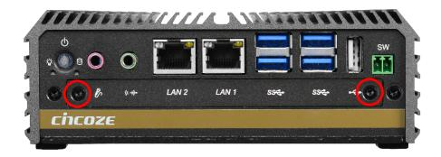
2. SIM card slot is at the front panel of the system.
