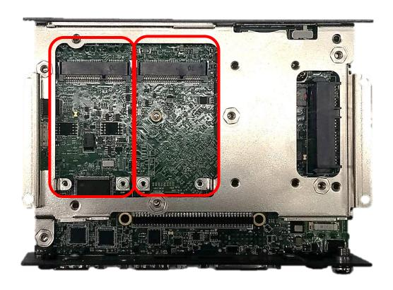
3. Tilt the Mini PCIe modules at 45 degree angle and insert it to the slot until the goldpated connector of module contacted firmly with the slot.
