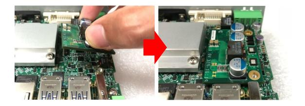
3. Turn over the heatsink and paste the thermal pad onto the marked by red squares.
