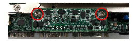
3. Attach the CMI-DIO bracket, and fasten 2 screws as marked on photo.
