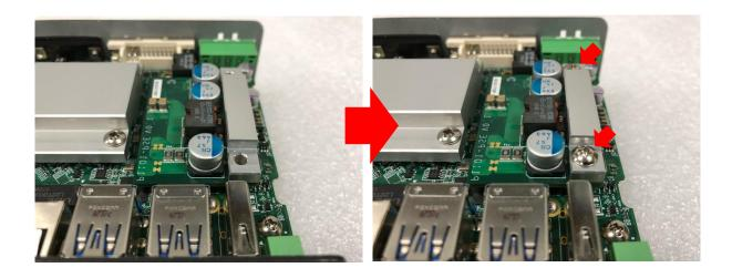
5. Paste the thermal pads onto the heatsink and coil carefully.
