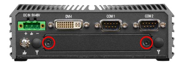
2. Insert CMI-HD module vertically to the female connector on the system's mainboard, and fasten 2 screws to fix it.
