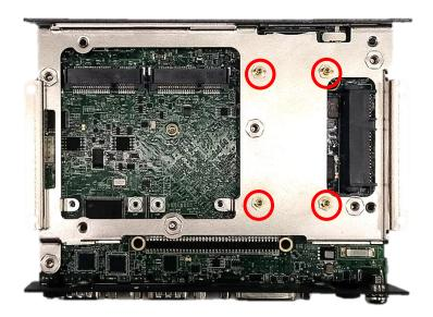
3. Connect the Half Slim SSD to the SATA connector of the unit and fasten the 4 screws.
