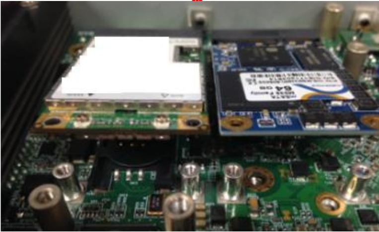
4. Press down the module and use the two screws to fix the module.
