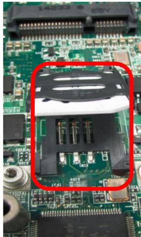
3. Press down the socket of SIM card to lock the location.
