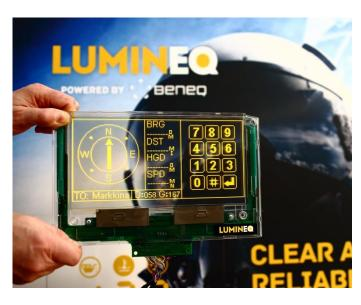
The ELT256.120.90 is a TASEL® transparent matrix display designed for use in applications requiring full see-through properties of the display, be that for functional or aesthetic reasons.
