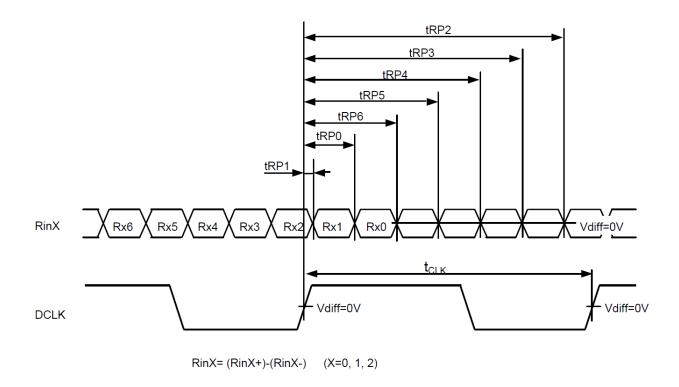
Figure 8. LVDS receiver timing chart.
