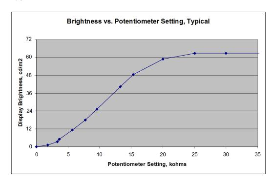
Figure 11. Analog dimming adjustment
