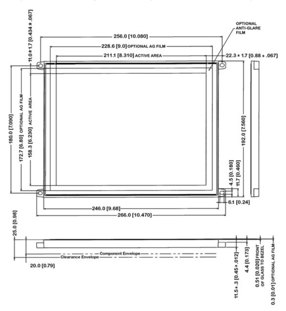
Dimensions are in millimeters; inches in brackets. Tolerances unless otherwise stated  $\pm 0.2$  mm
