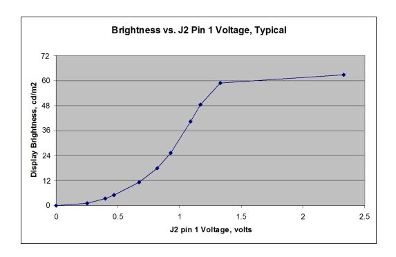
Figure 12. External voltage dimming
