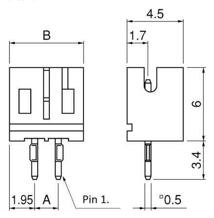
Figure 10. Dimming connector J2
