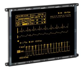
EL640.480-AM LVDS is a VGA-display for use in extreme operating conditions.
