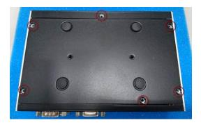
Step 2 Remove 4x rubber pad as shown.
