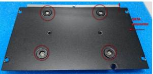
Step 4 Connect SATA and power cable with HDD/SSD as shown.
