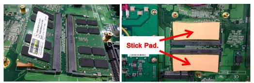
Step 9 Secure DRAM cover and install the internal bracket, front bezel. Fasten the all screws to complete the installation.
