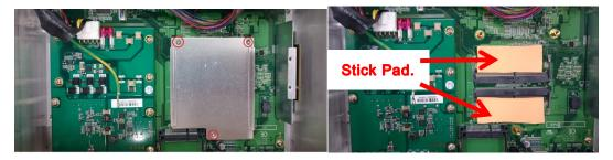
Step 8 Install the DDR cautiously and put on the thermal again.
