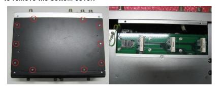
One slot contains an internal SIM card slot which can support 2G/3G/4G modules.
