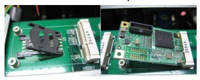
Step 4 Fasten the screws to complete the installation.
