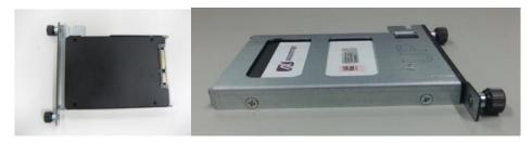
Step 3 Install CFast and SATA drive to the slot.
