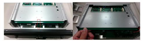
Step 7 Loosen below screws to remove cover and put on the thermal pad.
