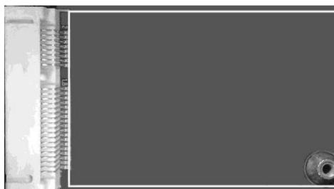
A PCI Express Mini Card can be applied to either PCI Express or USB 2.0. The USB 2.0 support will be helpful during the transition to PCI Express, because peripheral vendors will need time to design their chipsets to have the PCI Express function. During the transition, PCI Express Mini Cards can be quickly implemented by using USB 2.0.
