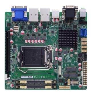
The MANO522 Mini-ITX motherboard supports the new 14nm 8<sup>th</sup> Generation Intel<sup>®</sup> Core<sup>™</sup> i7/ i5/ i3 and Pentium<sup>®</sup> processors in LGA1151 package. Featuring the new Intel<sup>®</sup> H310 Express chipset with two DDR4 2400/2666MHz memory support, this motherboard is built to perform best stability and reliability for industrial applications.
