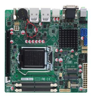
The MANO520 Mini-ITX motherboard supports the new 14nm 8<sup>th</sup> Generation Intel<sup>®</sup> Core ™ i7/ i5/ i3 and Pentium<sup>®</sup> processors in LGA1151 package. Featuring the new Intel<sup>®</sup> H310 Express chipset with two DDR4 2400/2666MHz memory support, this motherboard is built to perform best stability and reliability for industrial applications.
