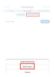
Step 4. Insert a USB disk to USB port. the USB disk that included full face photos (front view) in .png or .jpg format with minimum resolution 640\*480. Use registrants' names for photo file names.
