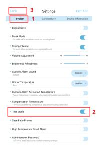
Step 2. Then click the "BACK" icon on the upper left corner to return scan temperature page and Display detailed temperature related parameters and distance
