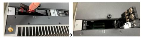
Step 5 Insert the HDD into the HDD tray.
