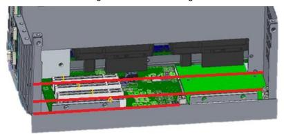
Slot 1~2: max. length up to 312mm
