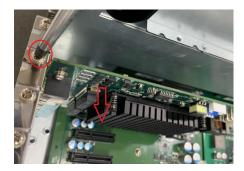
**Step 6** Fasten the below bracket in chassis with standard height (111mm) add-in cards.
