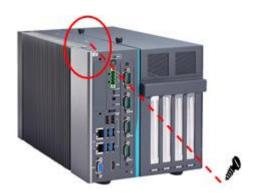
**Step 4** Insert the wireless LAN card into the slot and push it down firmly. Then screw the card tightly to the mainboard.
