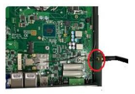
Note:Please use the supplied extended bracket when using a half-size Mini card
