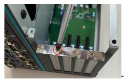
**Step 5** Align the PCI or PCIe card with the slot, press the card into the slot until it is firmly seated and screw it.
