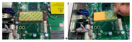
**Step 6** Insert the SSD card to slot and push it down firmly. Then screw the card tightly to the mainboard.
