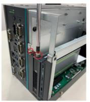
Step 11 Insert the air duct bracket's metal part as marked B below and screw the 4 screws.
