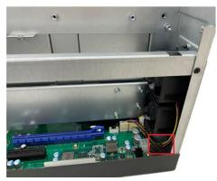
Step 8 Remove the slot brackets.
