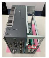
Align the PCI or PCIe card with the slot, press the card into the slot until it is firmly Step 5 seated and screw it. Then, plug the graphics card power cable.
