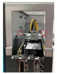
**Step 10** Close the cover back to the chassis and fasten the screw. The installation is complete.
