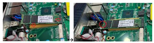
**Step 7** Paste the other thermal pad on the module and then remove the protective film, as illustrated below.
