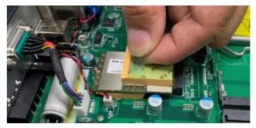
**Step 8** Remove the antenna plugs from the top of the back cover, install the antennas on the antenna connectors as marked in the illustration below, and then insert the SIM card into the SIM slot.
