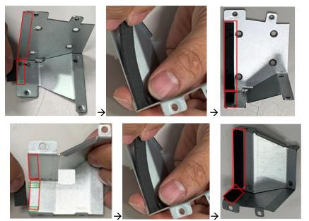
**Step 4** Paste the 4 poron pads on air duct brackets, as illustrated below.
