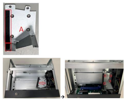
**Step 10** Align the T4 card with the slot, press the card into the slot until it is firmly seated, and screw the T4 card bracket and slot bracket to the chassis.
