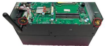
Step 7 Close the cover back to the chassis and fasten all screws. The installation is complete.
