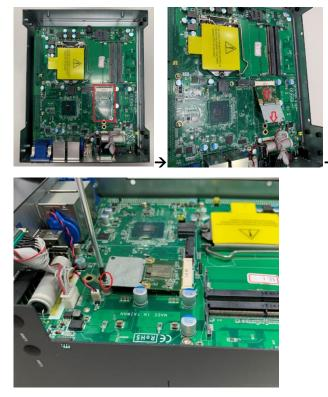
Step 6 Remove the antenna plugs from the top of back cover, and then install the antennas on the antenna connectors.
