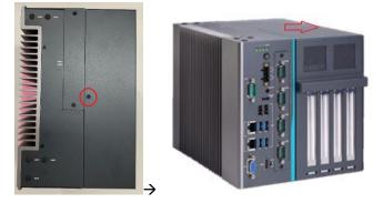
Step 4 Locate the PCI or PCIe slots and remove the slot bracket from the slot in which you want to add the card.
