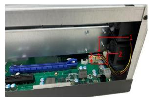
Step 7 Route the cables and put the cables in red mark area, as illustrated below.
