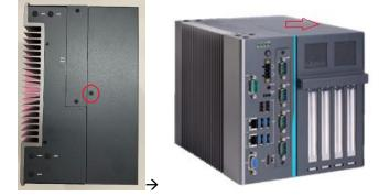
**Step 5** Unscrew the bracket, fasten the fan module into the expansion box and plug cable(s) to connector(s).
