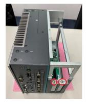
**Step 9** Insert the air duct bracket's metal part as marked A below and screw the 4 screws.
