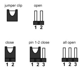
Before applying power to IMB211 Series, please make sure all of the jumpers are in factory default position. Below you can find a summary table of all jumpers and onboard default settings.
