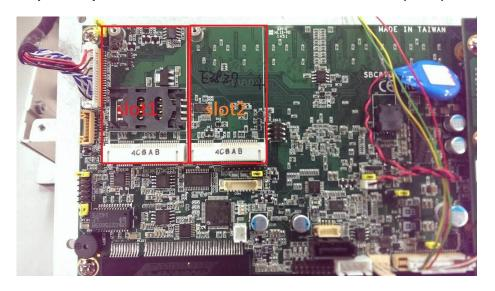
Step 2 Insert a wireless LAN card to slot 1. Screw it firmly on the slot.
