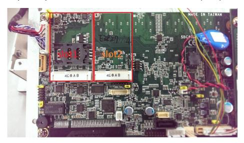
Step 2 Insert an mSATA card to slot 2. Screw it firmly on the slot.
