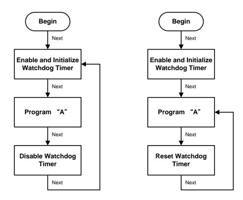
WDT Sample Program Enable WDT 1.Enable configuration -O 2E 87 -O 2E 87 2. Select Logic device: -O 2E 07 -O 2F 08 3. WDT Device Enable -O 2E 30 -O 2F 01 4. Set timer unit -O 2E F0 -O 2F 00 -> (00: Sec; 08: Minute) 5. Set base timer: -O 2E F1 -O 2F 0A → Set Reset Time (Ex.0A:10 Sec) **Disable WDT** 1.Enable configuration -O 2E 87 -O 2E 87 2. Select Logic device: -O 2E 07 -O 2F 08 3. WDT Device Disable -O 2E 30 -O 2F 00
