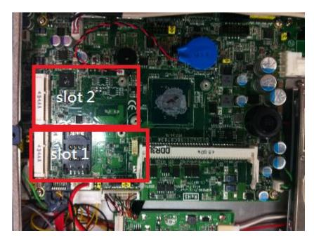
Open the back cover and find out the mini-card slot on main board. Step 1
