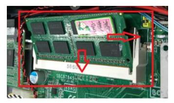
Step 3 Install the memory module into the socket and push it firmly down until it is fully seated. The socket latches are levered upwards and clipped on to the edges of the DIMM.
