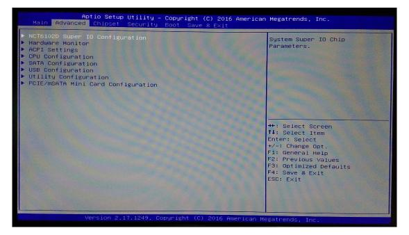
The Advanced menu allows users to set configuration of the CPU and other system devices. You can select any of the items in the left frame of the screen to go to the sub menus:
