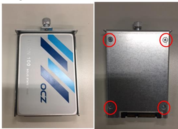
Figure 2-5 Fasten the four screws
