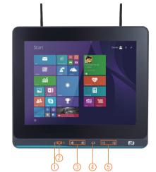
1. Power LED 2. HDD LED 3. Brightness adjust +/-4. Display on/off 5. Volume on/off
