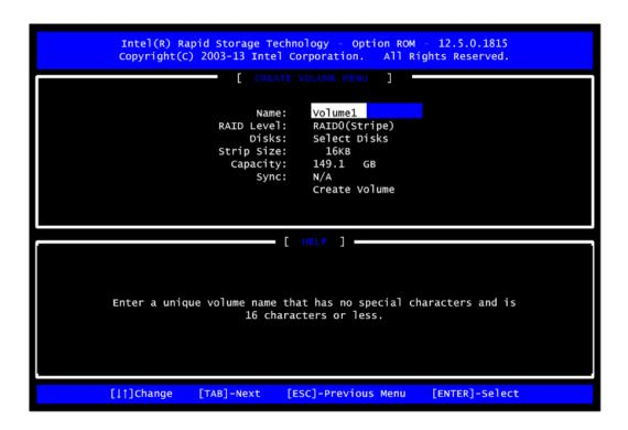
3.4. When finished, press <Enter> to select a RAID level. There are three RAID levels: RAID0, RAID1 and RAID5 and RAID10. Select a RAID level and press <Enter>.
