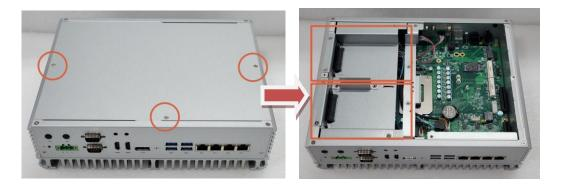
Step 3 Assembly each SSD/HDD with the HDD bracket with 2 screws.
