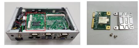
Step 5 Holding the Wi-Fi PCI Express mini card at a 45 degree angle up from horizontal; slowly insert the golden fingers into the PCI Express slot until it is fully inserted in and fasten screws and connect the cable to antenna.
