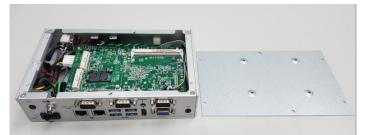
Step 4 Locate the DDR3L SO-DIMM slot, holding the DDR3L SO-DIMM at a 30 degree angle up from horizontal; slowly insert the golden fingers into the DDR3L SO-DIMM slot until it is fully inserted in.
