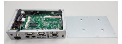
Step 4 Locate the PCI Express mini card slot on the board and prepare the Wi-Wi mini card and bracket from the min card accessory pack.
