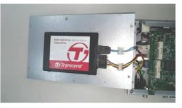
Note: Please notice the direction of connector for HDD/SSD.
