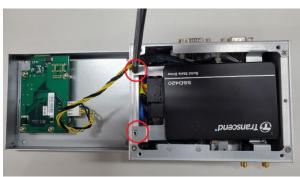
Step 6 Put the bottom cover back and fasten all of screws.
