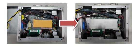
Step 7 Put the bottom cover back and fasten all of screws.
