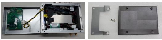
Step 4 Assembly the SSD/HDD with the two HDD mounting screws and connect the SATA cable. Be sure the PCB side of the SSD/HDD facing to left.
