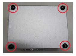
Step 3 Open the bottom cover and prepare the SSD/HDD and bracket from the accessory box.
