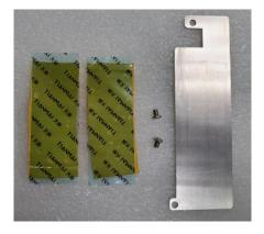
Step 5 Put the thermal pad on both up and down side of the DRAM.
