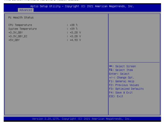
This screen displays the temperature of system and CPU, system voltages (VBAT, +3.3V, +3.3V standby and +5V).
