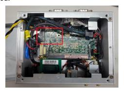
Step 4 Insert the M.2 Wi-Fi module firmly and fasten the screw, then connect the cable.
