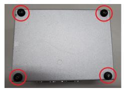
Step 3 Open the bottom cover and Locate M.2 2230 key E connector within the red line as marked.
