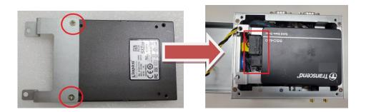
Step 5 Fasten the HDD/SSD bracket into the chassis.
