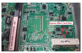
Step 5 Slide Mini Card into Mini Card slot with caution, and fasten screw of Express Mini Card.
