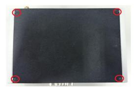
Step 3 Remove the HDD bracket then find Mini Card location.
