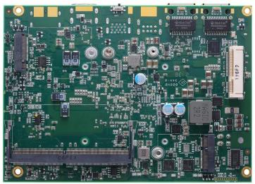
The CAPA322 is a 3.5" embedded board with Intel® Celeron® processor J6412 and N6210 & Atom® x6413E processor that deliver outstanding system performance through high-bandwidth interfaces, multiple I/O functions for interactive applications and various embedded computing solutions.
