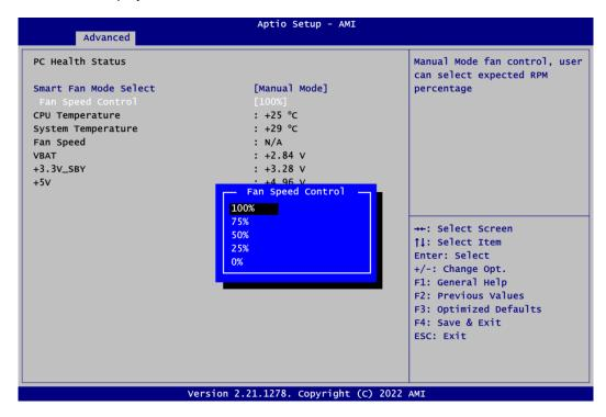
This screen displays the temperature of system and CPU, fan speed in RPM and system voltages (VBAT, +3.3V\_SBY and +5V).
