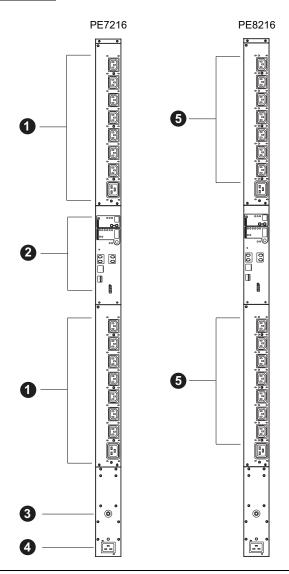
**Note:** The PE7216 / PE8216 unit components are identical except for the outlet LEDs — the PE7216 has none while the PE8216 has 16, as shown by number 5 above.
