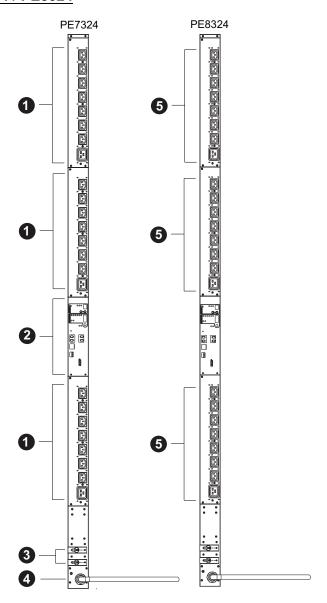
**Note:** The PE7324 / PE8324 unit components are identical except for the outlet LEDs — the PE7324 has none while the PE8324 has 24, as shown by number 5 above.
