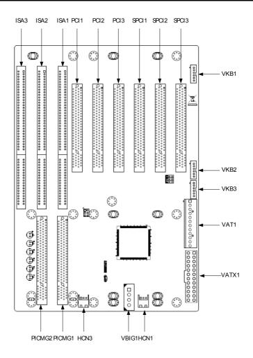
Note: When a PCI card is inserted in PCI1, it may conflict with the CPU card.
