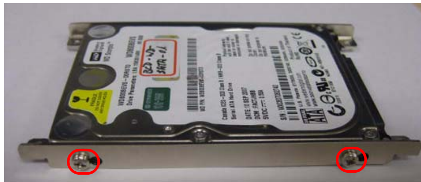
Figure 1.9 Fasten Screws on the SATA HDD Bracket
