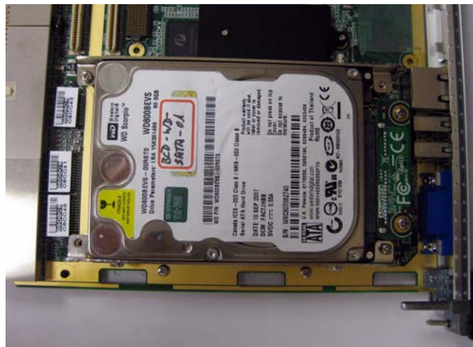
Figure 1.10 Insert SATA HDD into SATA Connector
