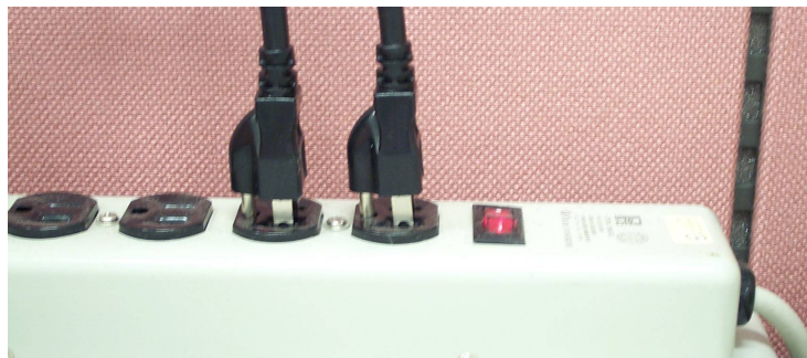
Figure 3.4: Power cord plugs should have same orientation in the socket/ 插座上电源线方向相同 / 插座上的電源線方向應相同
