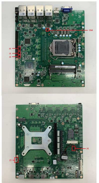
Figure 2.1 Jumper Layout
