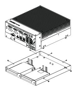
1. Unscrew six screws on the bottom cover.
