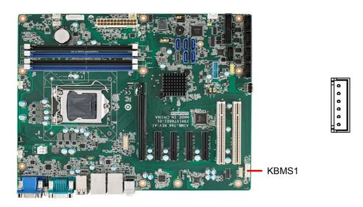
A 6-pin header on the motherboard is for an optional PS/2 keyboard/mouse cable. This gives system integrators greater flexibility in designing their systems.
