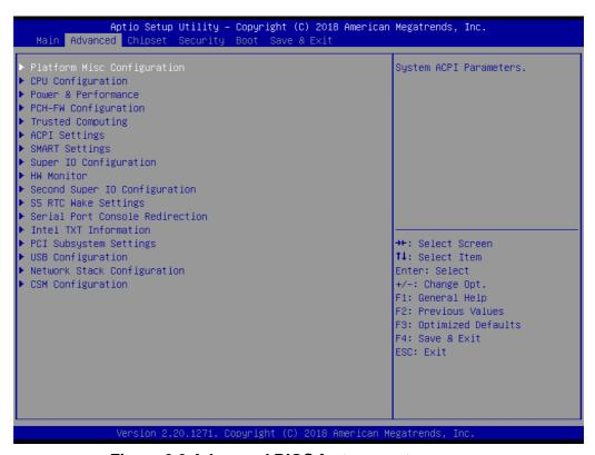
Figure 3.3 Advanced BIOS features setup screen
