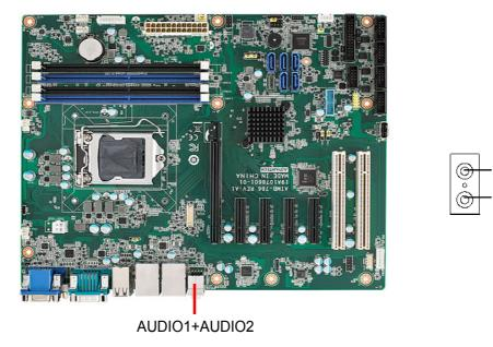
Line Out can be connected to external audio devices like speakers or headphones. Mic In can be connected to a microphone.
