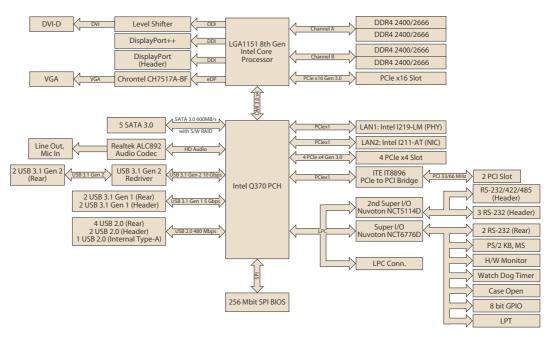
Figure 1.3 Block Diagram
