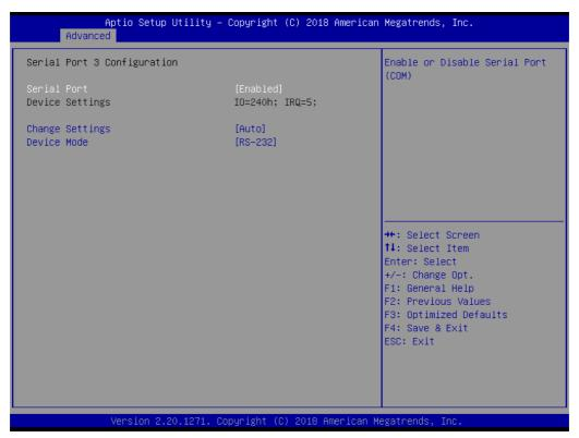
Figure 3.25 Serial Port 3 Configuration
