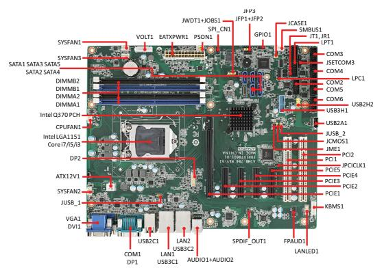
**Figure 1.1 Jumper and Connector Locations**
