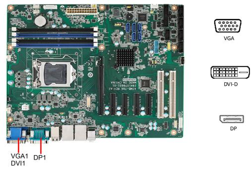
The AIMB-786 includes VGA, DVI-D, and DisplayPort interface that can connect display devices. Pin assignments are detailed in Appendix B.
