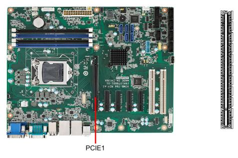
The AIMB-786 provides a PCIe x16 slot for users to install an add-on peripheral card for extension requirements.
