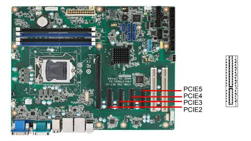
The AIMB-786 offers four PCIe x4 slots for users to install add-on cards for extension requirements.
