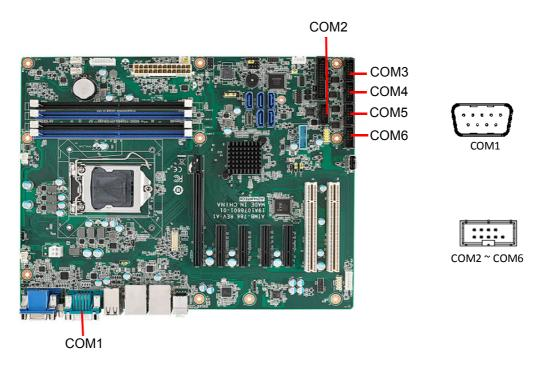
The AIMB-786 offers six serial ports (one on the rear panel and five onboard). COM3 can be configured as RS-232/422/485 by jumper settings (see Chapter 1), and selecting correct device mode for RS-485 under BIOS is necessary (see Chapter 3). These ports can connect to a serial mouse, printer or communications network. The IRQ and address ranges for those ports are fixed. However, if you want to disable the port or change these parameters later, you can do this in the system BIOS setup. Dif-
