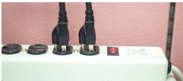
Figure 3.7 Power Cord Plugs Should Have Same Orientation in Socket/ 插座上电源线方向相同 / 插座上的電源線方向應相同
