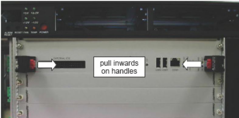
Figure 2-2: Latching the cPCI module handles securely.
