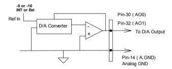
The operation of D/A conversion is more simple than A/D operation. You only need to write digital values into the D/A data registers and the corresponding voltage will be output from the AO1 or AO2. Refer to section 4.9 for information about the D/A data registers. The mathematical relationship between the digital number DAn and the output voltage is formulated as following:
