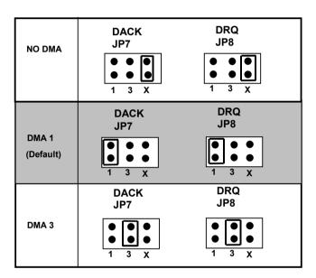
Figure 2.4 DMA Channel Setting
