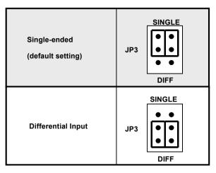
Figure 2.3 Analog Input Channels Configuration
