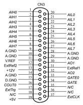
Figure 3.3b. Pin Assignment of CN3
