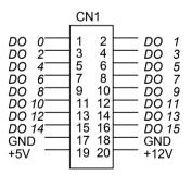
Figure 3.2. Pin Assignment of CN1
