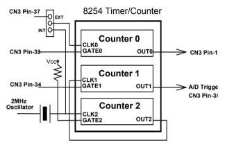
The clock source of counter 0 can be internal or external, while the gate can be controlled externally and the output is send to the connector CN3. As to counter 0 and counter 1, the clock source is internally fixed, while the gate can be controlled externally and the output is send to the connector CN3 too. All the timer/ counter signals are TTL compatible.
