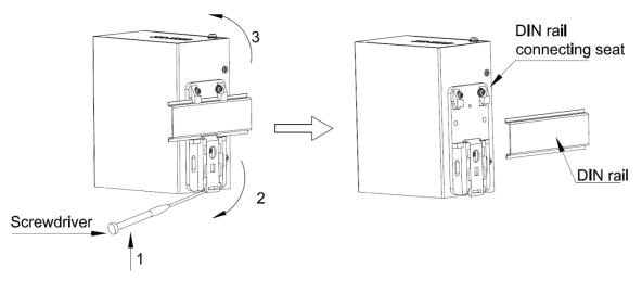
Figure 5 Disassemble from rail
