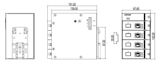
Figure 3 Dimensions (mm)
