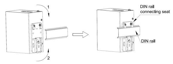
Figure 4 DIN rail chassis installation
