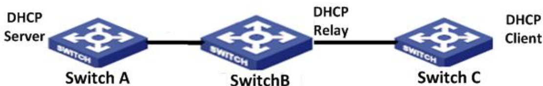
Figure 293 DHCP Typical Configuration Example
