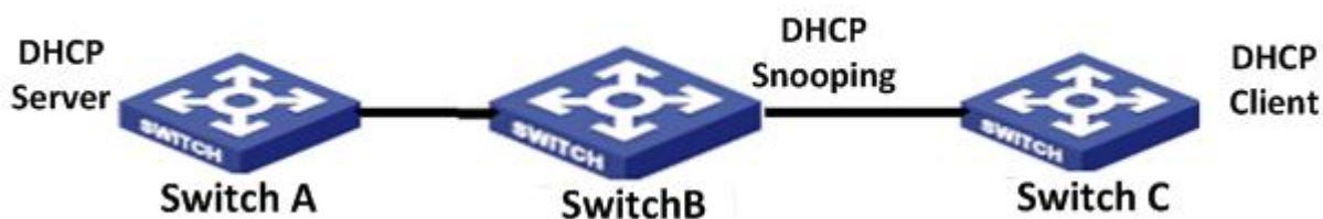
Figure 294 DHCP Typical Configuration Example
