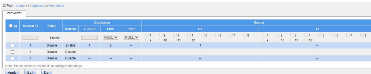
Figure 280 Configure Remote Port Mirroring
