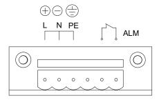
The power supply works with a wide range of input voltage, 110~220V AC/DC.
