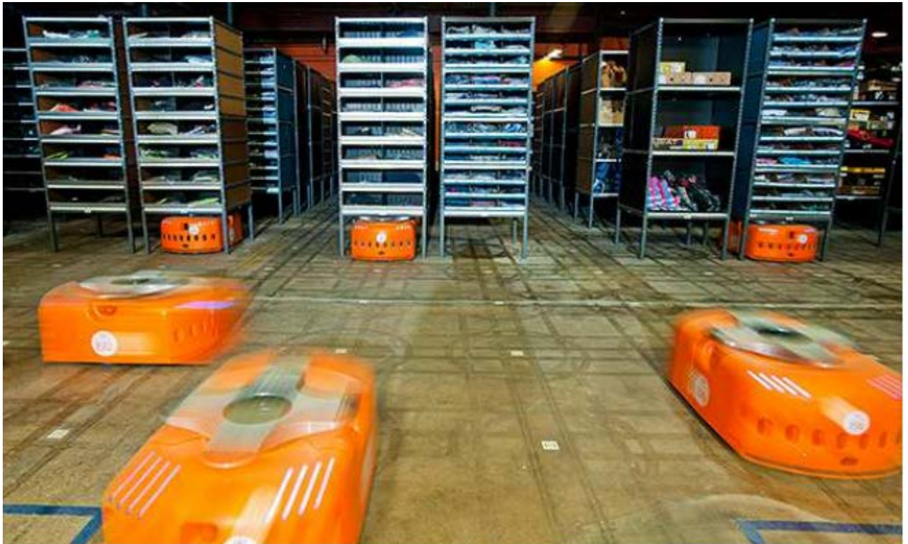
Figure 1-2 Working scenario of AGV
