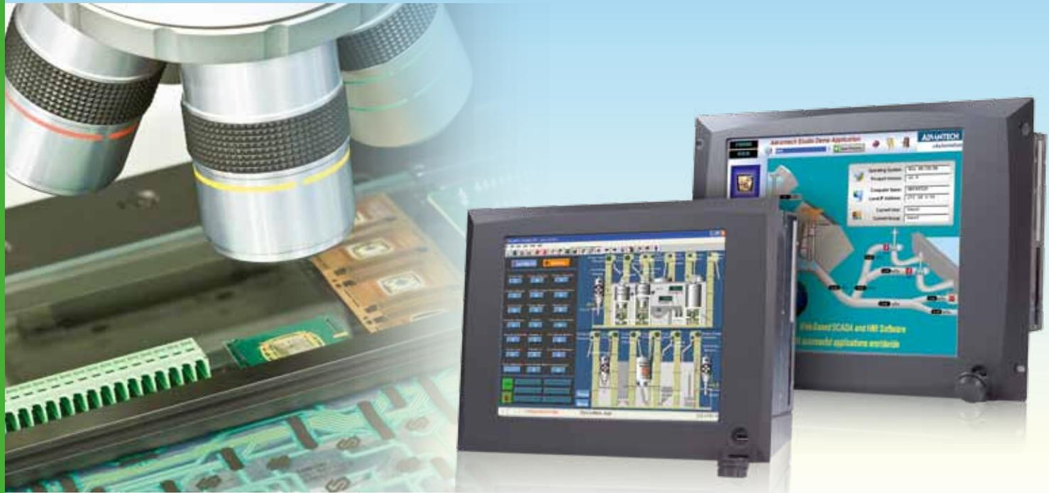
With latest Intel® Core™ i7 mobile processor, IPPC-9000 series provides high computing performance at the same time supports intelligent iManager with value-added APIs & runtime OS QNX. In addition, design with die-cast bezel and stainless steel housing makes it extremely rugged but compact. Positioned as a rugged & intelligent panel PC, IPPC-9000 series is suitable for monitor and control management or even complicated applications like surveillance systems.
