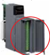
I-87018PW-G/S CR= I-87018PW connects CN-1824 directly
